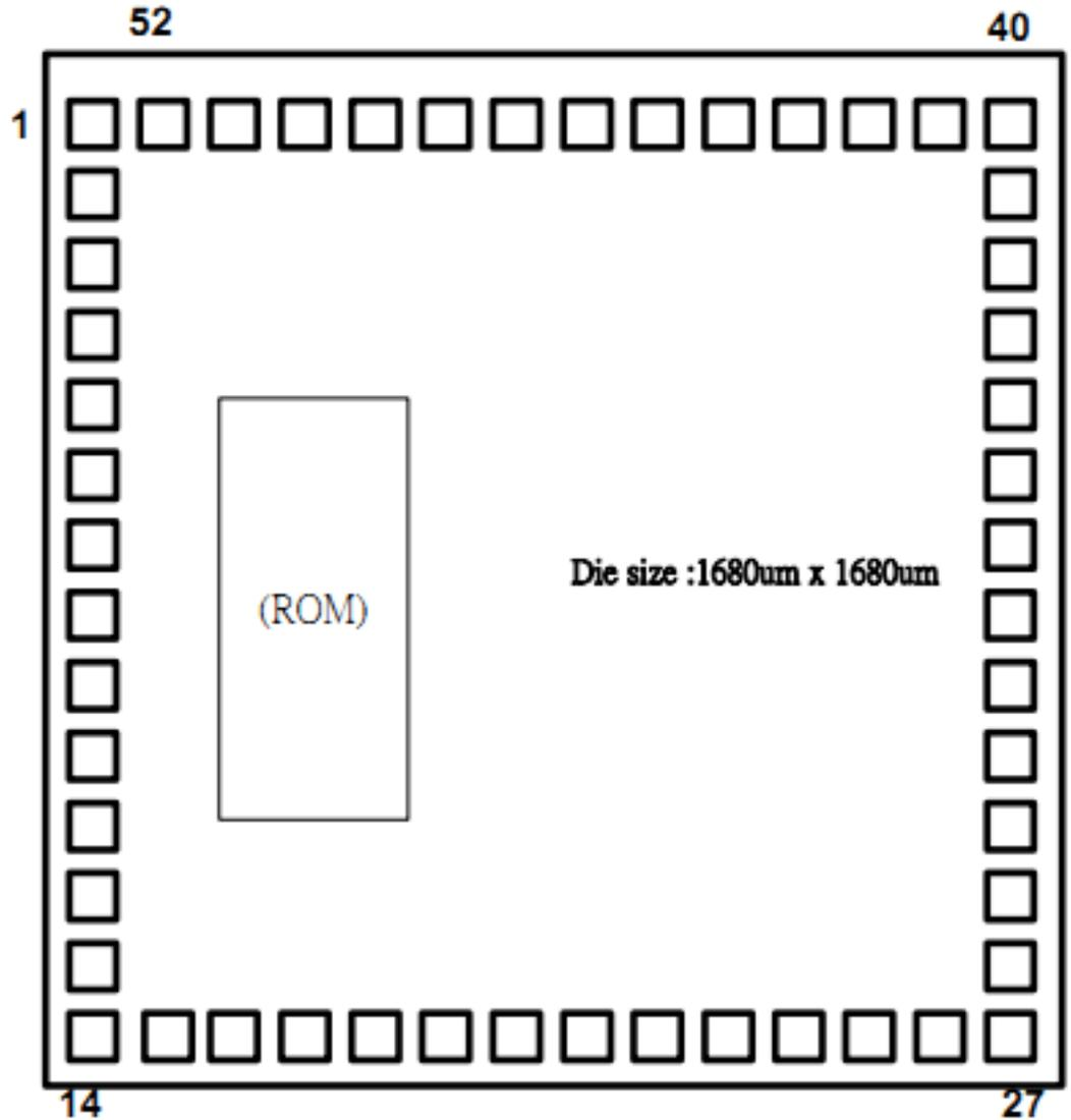
The substrate of chip should be connected to GND.
